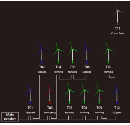
All alarms are archived in **Alarm History**. **Topography** view provides a graphical display of the communications fiber to provide insight into substation and fiber related issues.
